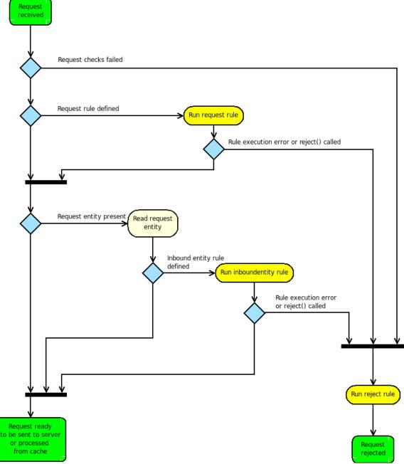
In the drawing, the observant reader will note that the green 'state' box in the lower left includes 'request ready to be processed from cache'. The current version of Yxorp does not define rules to run if a request is served from Yxorp's cache; this will be added in some future version.
