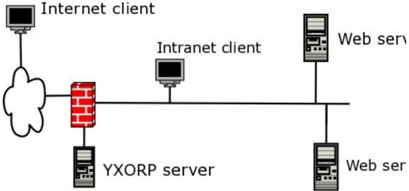
This setup is almost as secure as the two-firewall setup. The differences are mainly that the complexity of the firewall rules is increased, and that one wrong rule in the firewall could open up the internal network. In a corporate environment, you would want to prevent that; if you are just running Yxorp at home and are in control of all involved systems, the
