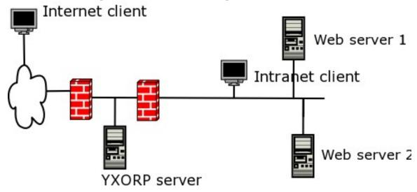
The difference with the minimal setup is that the traffic between Yxorp and the web servers is now restricted by the second firewall; this means that even if Yxorp is compromised, it is still not possible to use that vulnerability to reach the Intranet clients or other systems on the internal network (like your server running Samba and NFS for your MP3-collection).
